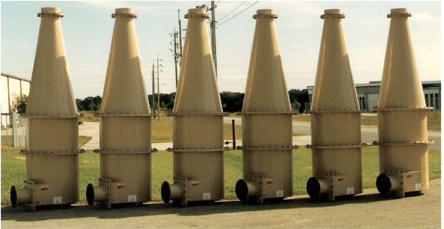
Six 24" cyclones with extended feed chambers for phosphate beneficiation.
